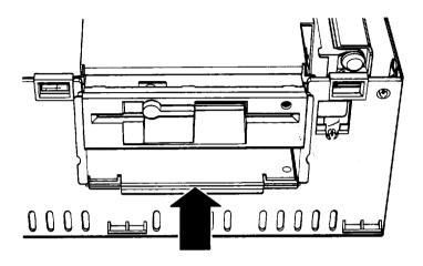
6. Locate the hard disk drive socket on the main system board (in front of the socket that holds the diskette drive ribbon cable). There is a notch on one side of the socket, as shown below.
